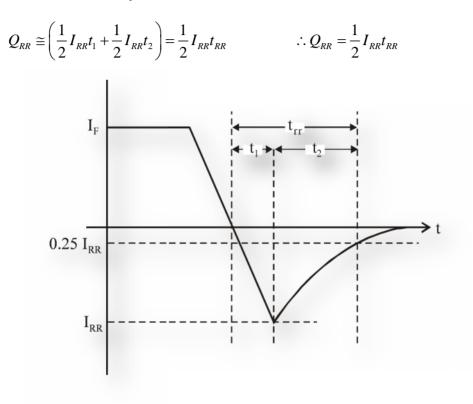
Fig 3 Reverse Recovery Characteristics
