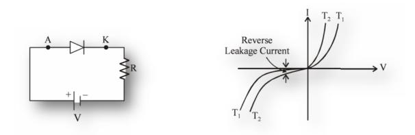
Fig 1 Diode Characteristics
