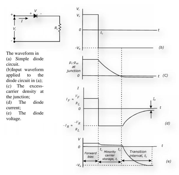
Fig 2: Storage & Transition Times during the Diode Switching
