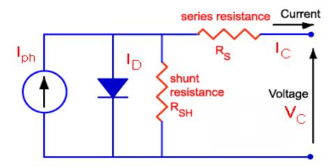
$$V_c = \frac{AkT_c}{e} \ln \left[\frac{I_{ph} + I_0 - I_c}{I_0}\right] - R_s I_c$$
